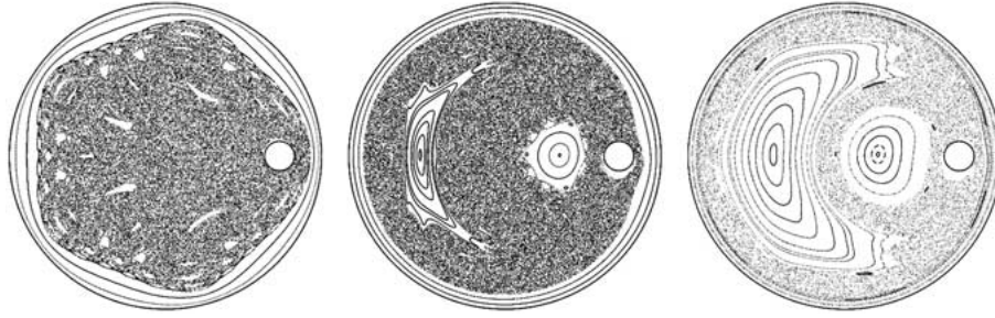
Figure 15. Iterated mappings, computed numerically, for the stirring protocols used in our experiments. From left to right the images correspond to the -4:1 , +4:1 and +6:1 stirring protocols.
