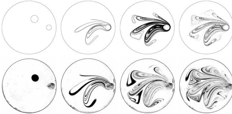
Figure 13. Comparison between numerical simulations (top row) and experiments (bottom row) using the -4:1 stirring protocol. The leftmost images show the initial (nominally) circular blob of radius 0.14a_{\text{out}} centred at the point (x, y) = (0.20, 0.30)a_{\text{out}} . The following snapshots show the blob after one, two and three complete stirring cycles.
