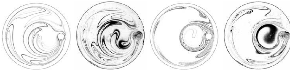
Figure 14. Further comparisons between numerical and experimental results. A circular blob of radius 0.14a_{\text{out}} placed at the centre of the outer cylinder was stirred for three cycles. The left-hand pair of images shows the results using the +4:1 protocol (numerical then experimental); the right-hand pair corresponds likewise to the +6:1 protocol.
